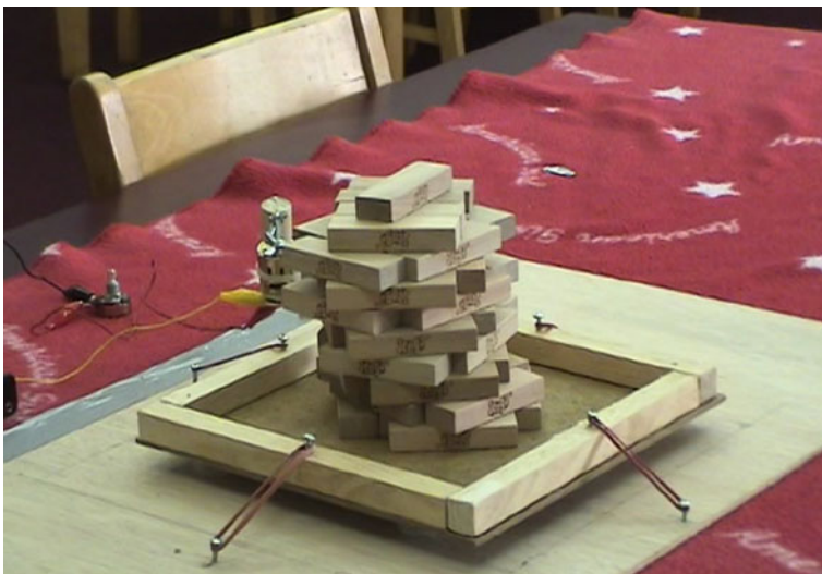
Fig. 1 Sample student-designed earthquake-proof structure on the earthquake simulator
